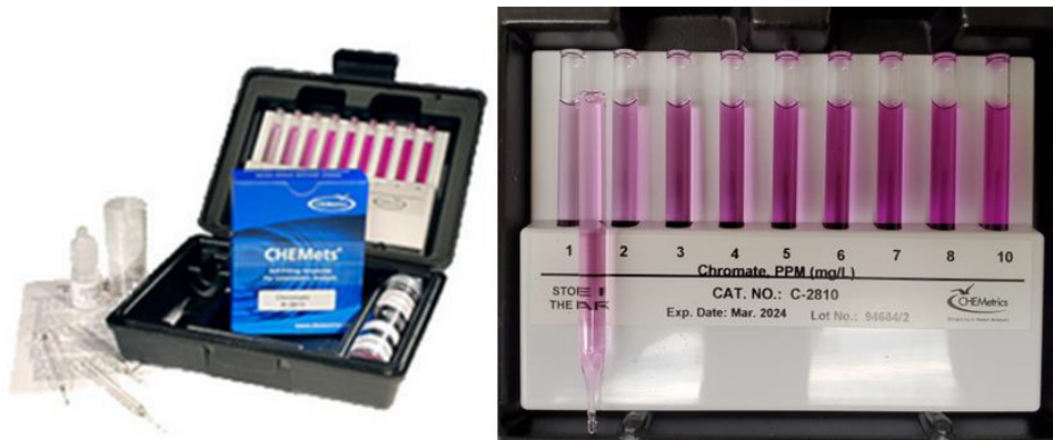
Figure 11 – CHEMetrics diphenyl carbazide (DPC) reaction-based Cr(VI) detection kit (left) and color comparator (right).
