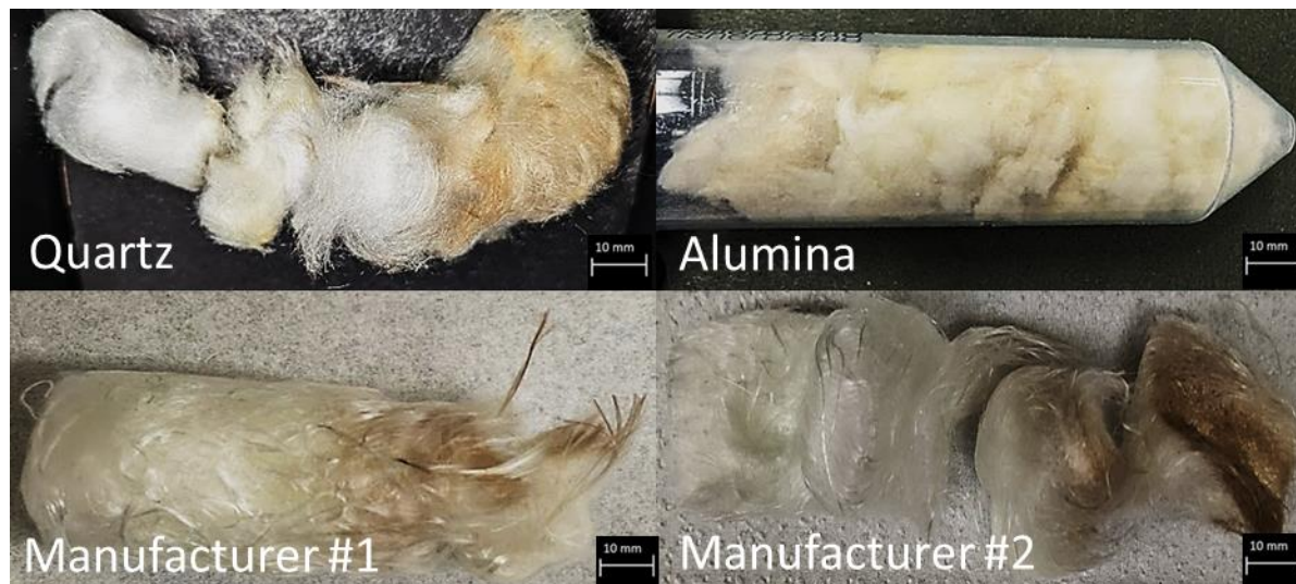
Figure 25: Fibers post-exposure for humid conditions, clockwise starting from top-left: quartz wool, alumina wool, insulation #1, and insulation #2.
