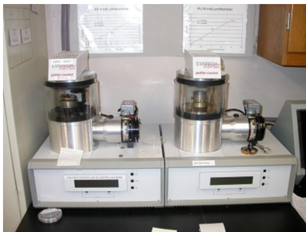
Figure 9 – Emitech K575X Peltier cooled metal coaters used for SEM sample preparation, located in Imaging and Chemical Analysis Lab (ICAL) at Montana State University.
