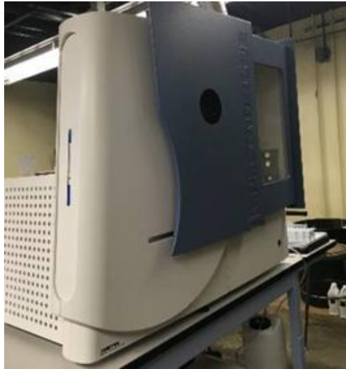
Figure 10 – SPECTROBLUE EOP TI Inductively Coupled Plasma Optical Emission Spectroscopy (ICP-OES) instrument located in Environmental Analytical Lab (EAL) at Montana State University.
