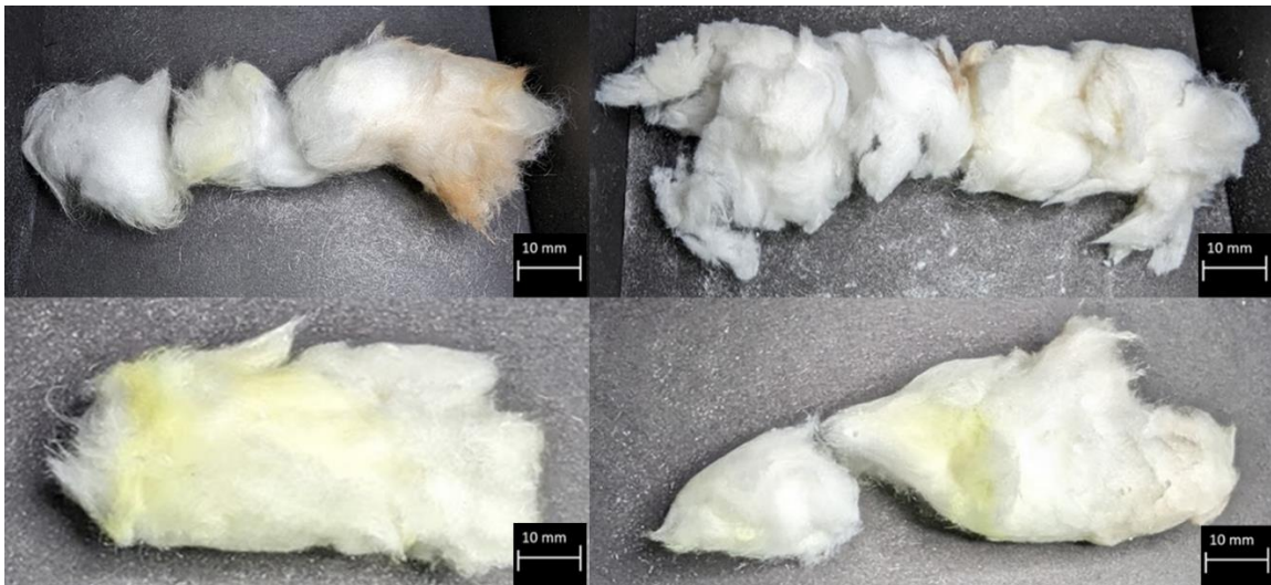
Figure 32: Ceramic insulating fibers post-exposure, counterclockwise from top left: quartz, AES #1, AES #2, and alumina wools.
