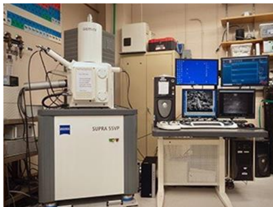
Figure 8 – Zeiss Supra 55VP Field Emission Scanning Electron Microscope (FE-SEM) with Energy Dispersive X-ray Spectroscopy (EDX) detector located in Imaging and Chemical Analysis Lab (ICAL) at Montana State University.
